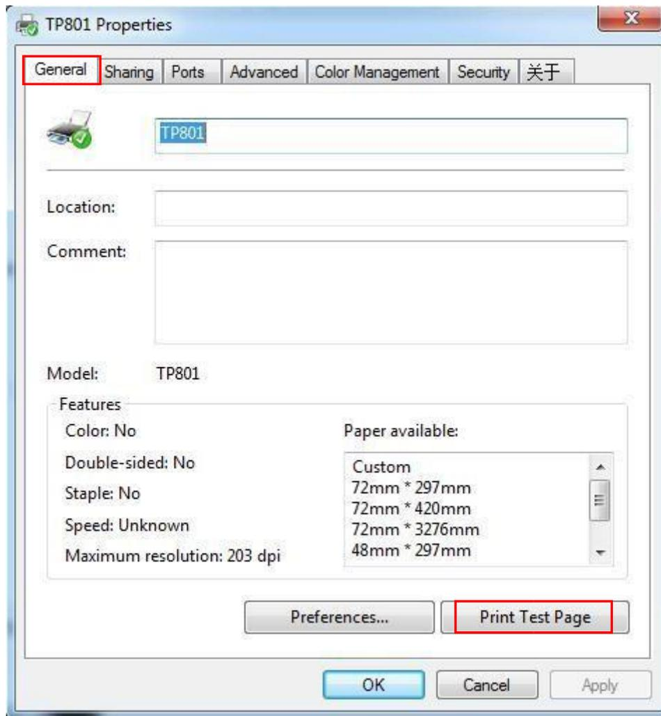
6. If the print test page can print normally, the following figure is displayed; if fails, check whether Bluetooth is disconnected or the corresponding COM port is occupied.
